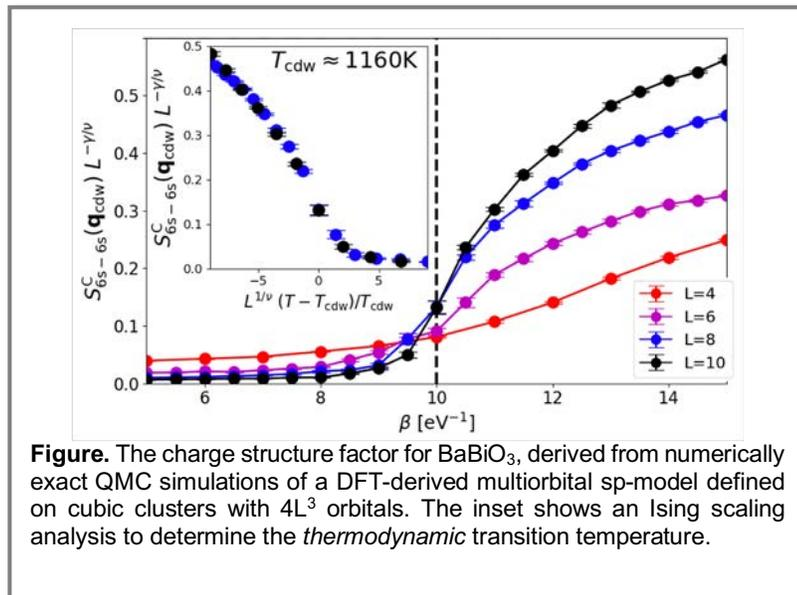
**Figure.** The charge structure factor for BaBiO<sub>3</sub>, derived from numerically exact QMC simulations of a DFT-derived multiorbital sp-model defined on cubic clusters with 4L<sup>3</sup> orbitals. The inset shows an Ising scaling analysis to determine the *thermodynamic* transition temperature.
