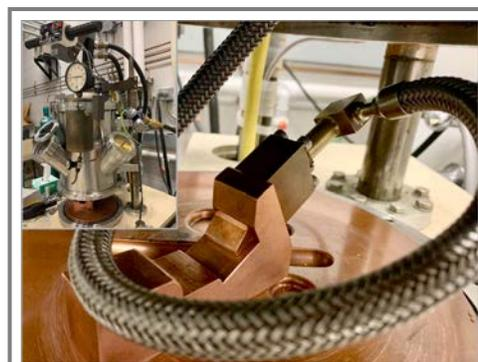
**Figure 2.** Anvil and hammer splat cooler to quench a liquid into an amorphous phase.
