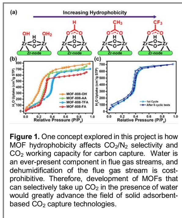
**Figure 1.** One concept explored in this project is how MOF hydrophobicity affects CO<sub>2</sub>/N<sub>2</sub> selectivity and CO<sub>2</sub> working capacity for carbon capture. Water is an ever-present component in flue gas streams, and dehumidification of the flue gas stream is cost-prohibitive. Therefore, development of MOFs that can selectively take up CO<sub>2</sub> in the presence of water would greatly advance the field of solid adsorbent-based CO<sub>2</sub> capture technologies.
