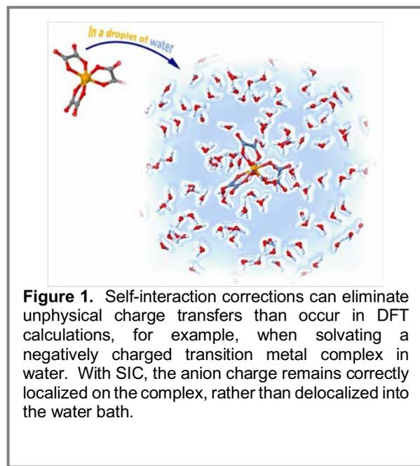
molecules. Other code-related initiatives include the first FLOSIC calculations for rare-earth (f-electron) atoms (Pederson, Baruah), which show significant improvement in FLOSIC orbital energies compared to electron removal energies, and a scheme to obtain a physically correct starting charge density in situations where DFT calculations give unphysical charge transfers (Pederson). Finally, the computationally efficient  $r^2$ SCAN functional was recently implemented in the FLOSIC code (Zope).
