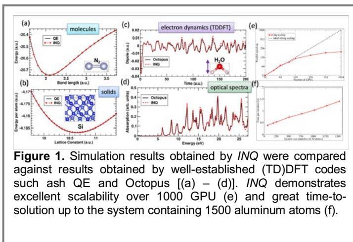
**Figure 1.** Simulation results obtained by *INQ* were compared against results obtained by well-established (TD)DFT codes such as QE and Octopus [(a) – (d)]. *INQ* demonstrates excellent scalability over 1000 GPU (e) and great time-to-solution up to the system containing 1500 aluminum atoms (f).
