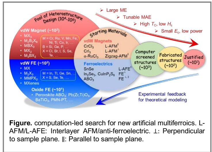
**Figure.** computation-led search for new artificial multiferroics. L-AFM/L-AFE: Interlayer AFM/anti-ferroelectric. ⊥: Perpendicular to sample plane. ||: Parallel to sample plane.
