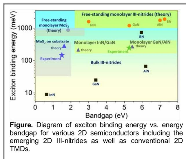
**Figure.** Diagram of exciton binding energy vs. energy bandgap for various 2D semiconductors including the emerging 2D III-nitrides as well as conventional 2D TMDs.
