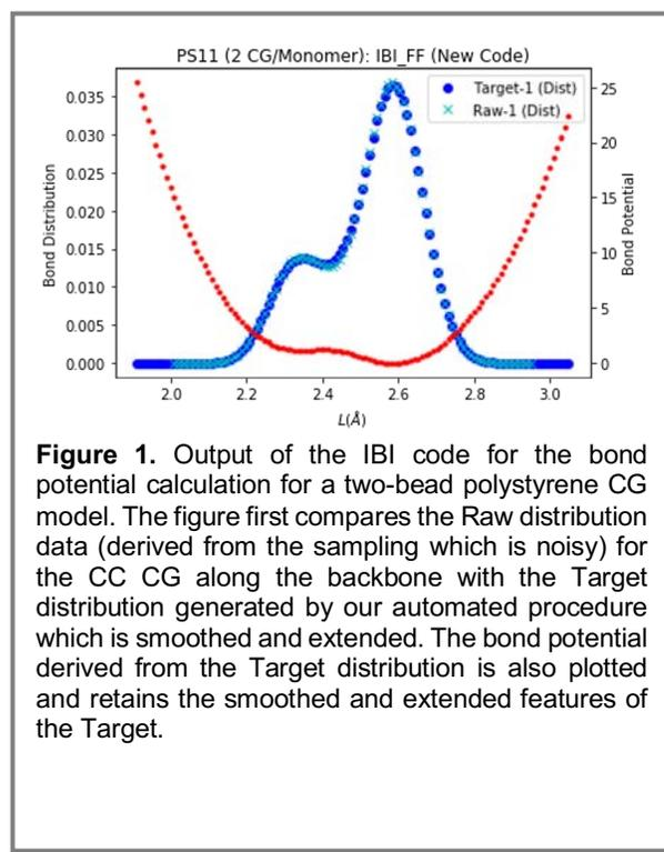
**Figure 1.** Output of the IBI code for the bond potential calculation for a two-bead polystyrene CG model. The figure first compares the Raw distribution data (derived from the sampling which is noisy) for the CC CG along the backbone with the Target distribution generated by our automated procedure which is smoothed and extended. The bond potential derived from the Target distribution is also plotted and retains the smoothed and extended features of the Target.
