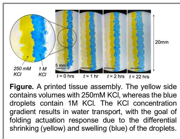
**Figure.** A printed tissue assembly. The yellow side contains volumes with 250mM KCl, whereas the blue droplets contain 1M KCl. The KCl concentration gradient results in water transport, with the goal of folding actuation response due to the differential shrinking (yellow) and swelling (blue) of the droplets.
