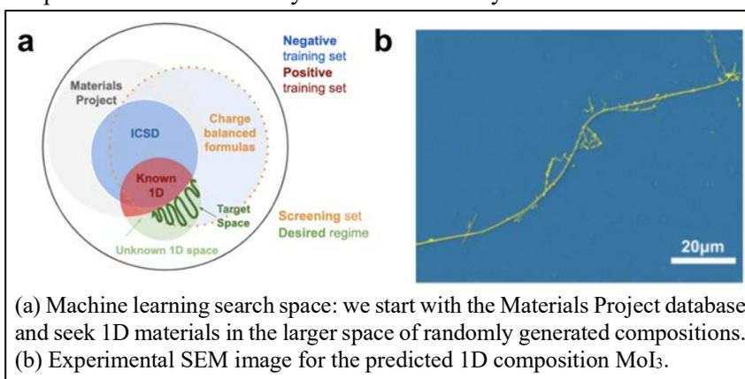
(a) Machine learning search space: we start with the Materials Project database and seek 1D materials in the larger space of randomly generated compositions. (b) Experimental SEM image for the predicted 1D composition  $\text{MoI}_3$ .
