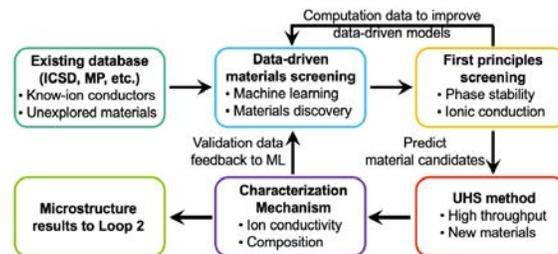
Figure 2. Scheme of Loop 1. Materials composition discovery by data-driven and first-principles
