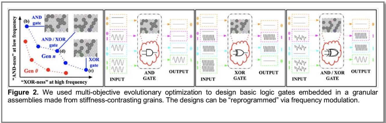
functionality of evolved assemblies by probing how they transform bits encoded as vibrations with zero or non-zero amplitude. We further compared the evolution of assemblies made of mass-contrasting particles and with assemblies made of stiffness-contrasting particles, and found that the latter were more evolvable.
