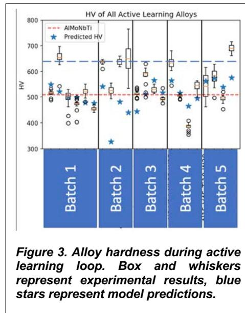
**Figure 3. Alloy hardness during active learning loop. Box and whiskers represent experimental results, blue stars represent model predictions.**
