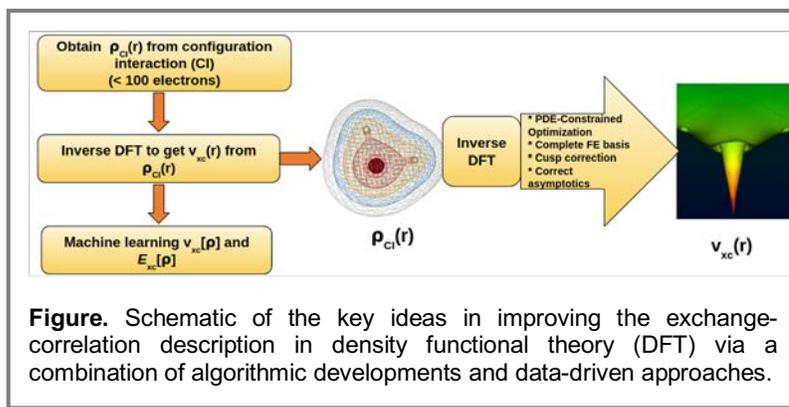
**Figure.** Schematic of the key ideas in improving the exchange-correlation description in density functional theory (DFT) via a combination of algorithmic developments and data-driven approaches.
