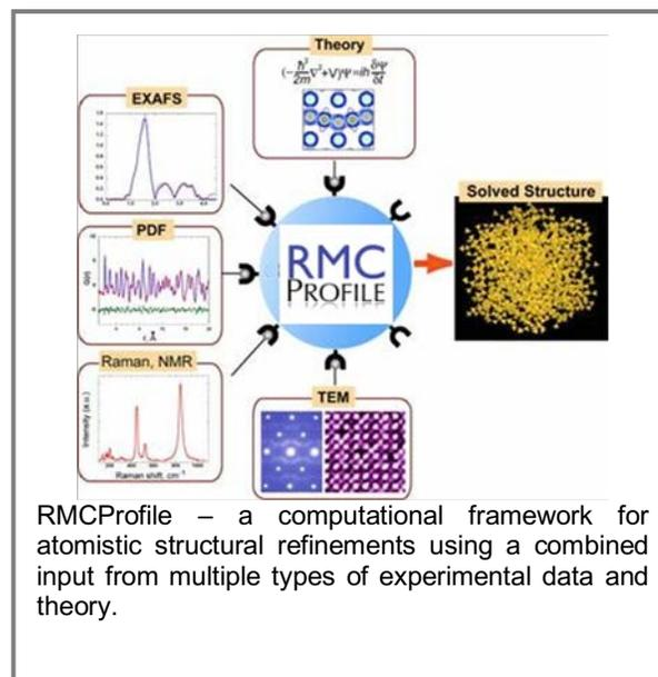
RMCProfile – a computational framework for atomistic structural refinements using a combined input from multiple types of experimental data and theory.
