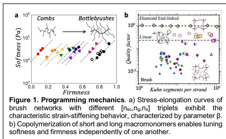
and fraction of the load-bearing strands. The decoded structures enabled classification of various polymer networks according to the effectiveness of stress distribution characterized by a topological quality factor (**Fig. 1b**).
