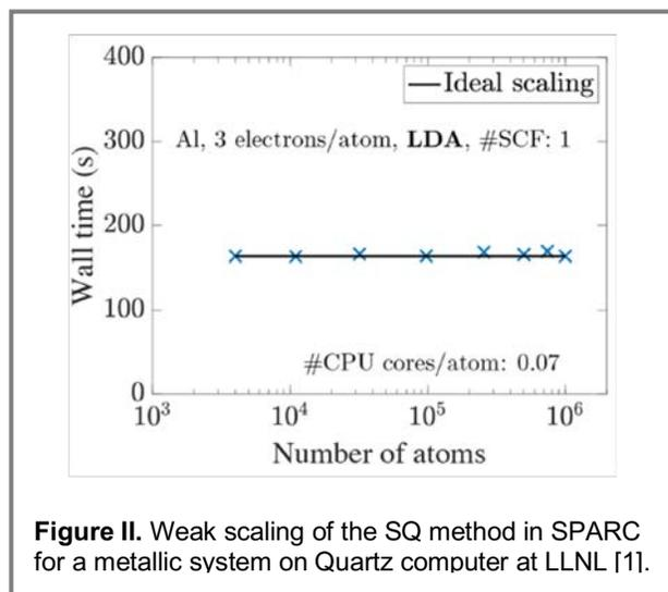
**Figure II.** Weak scaling of the SQ method in SPARC for a metallic system on Quartz computer at LLNL [1].
