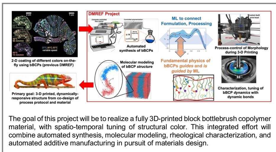
The goal of this project will be to realize a fully 3D-printed block bottlebrush copolymer material, with spatio-temporal tuning of structural color. This integrated effort will combine automated synthesis, molecular modeling, rheological characterization, and automated additive manufacturing in pursuit of materials design.
