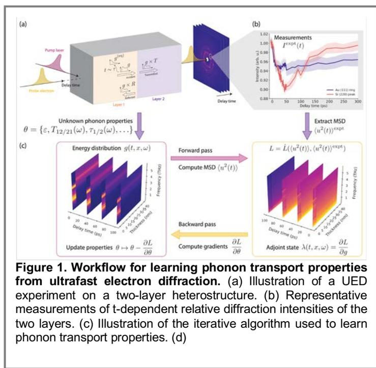
**Figure 1. Workflow for learning phonon transport properties from ultrafast electron diffraction.** (a) Illustration of a UED experiment on a two-layer heterostructure. (b) Representative measurements of t-dependent relative diffraction intensities of the two layers. (c) Illustration of the iterative algorithm used to learn phonon transport properties. (d)
