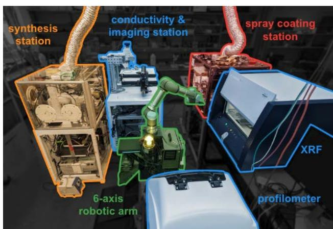
**Figure 1:** Ada is a self-driving laboratory that makes and tests thin-film materials. It consists of a robotic arm surrounded by various material synthesis, processing, and characterization stations.
