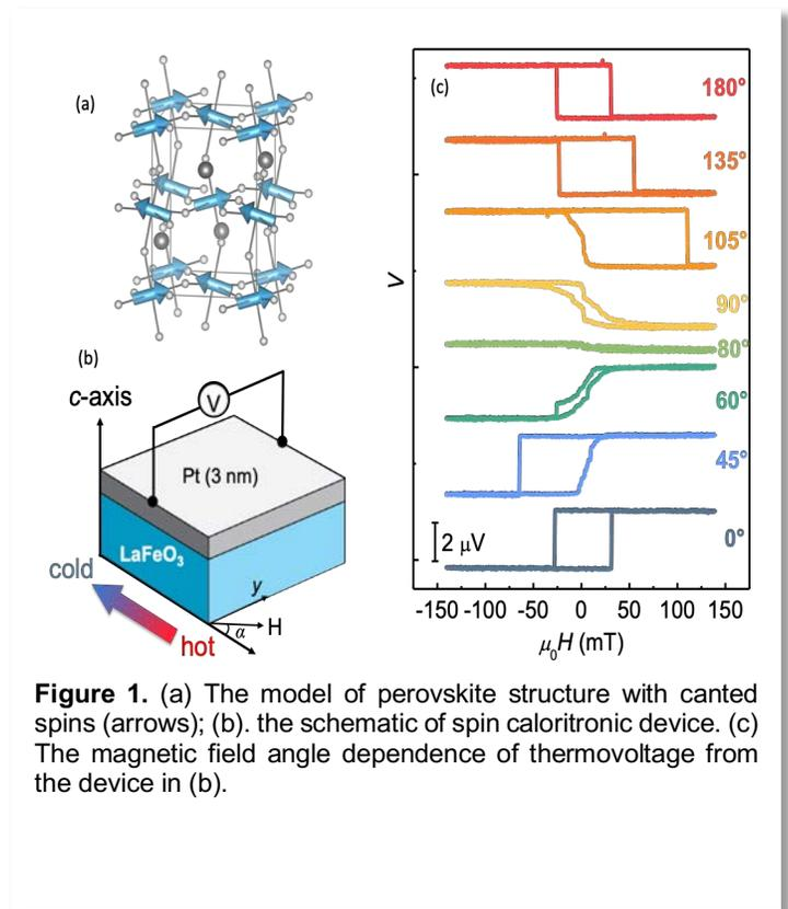
**Figure 1.** (a) The model of perovskite structure with canted spins (arrows); (b) the schematic of spin caloritronic device. (c) The magnetic field angle dependence of thermovoltage from the device in (b).
