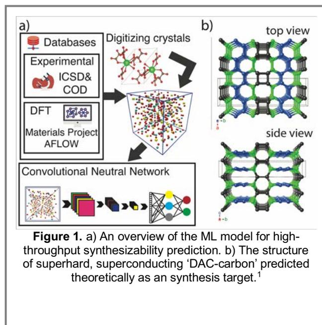
**Figure 1.** a) An overview of the ML model for high-throughput synthesizability prediction. b) The structure of superhard, superconducting 'DAC-carbon' predicted theoretically as a synthesis target.<sup>1</sup>
