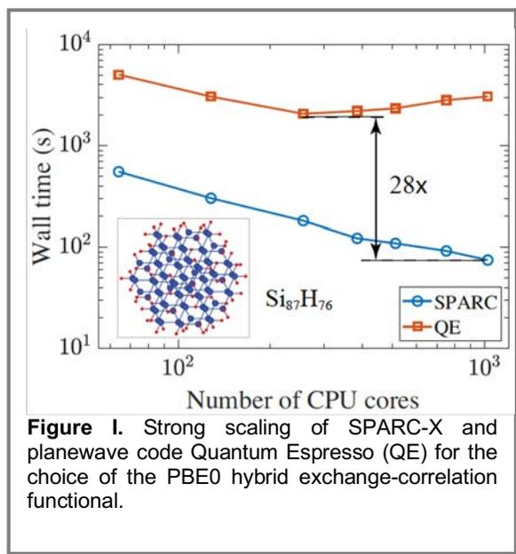
**Figure I.** Strong scaling of SPARC-X and planewave code Quantum Espresso (QE) for the choice of the PBE0 hybrid exchange-correlation functional.
