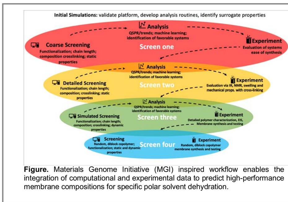
**Figure.** Materials Genome Initiative (MGI) inspired workflow enables the integration of computational and experimental data to predict high-performance membrane compositions for specific polar solvent dehydration.
