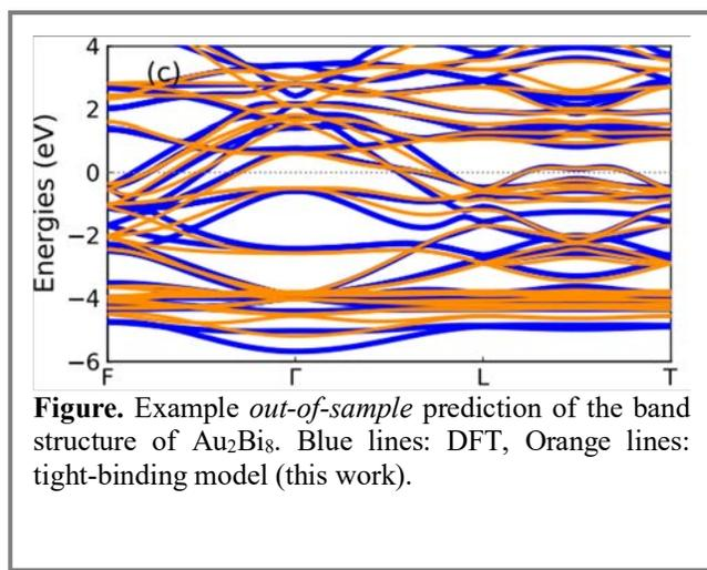
**Figure.** Example *out-of-sample* prediction of the band structure of  $\text{Au}_2\text{Bi}_8$ . Blue lines: DFT, Orange lines: tight-binding model (this work).
