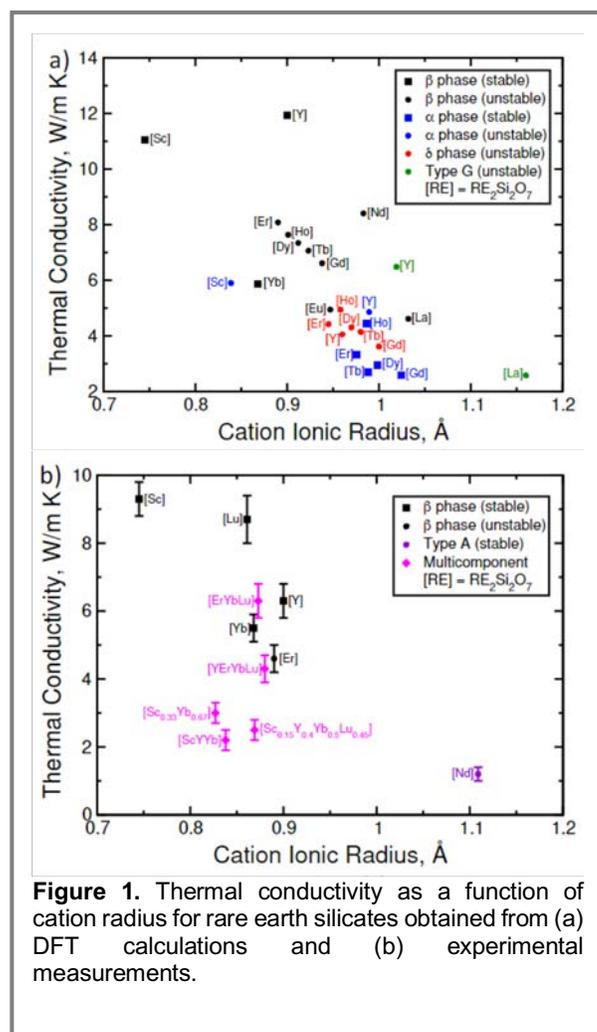
**Figure 1.** Thermal conductivity as a function of cation radius for rare earth silicates obtained from (a) DFT calculations and (b) experimental measurements.
