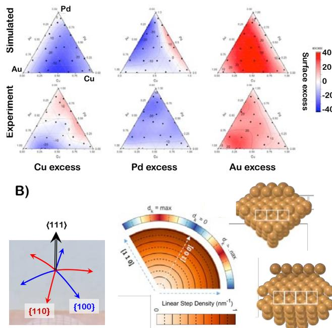
Figure 1. A) Segregation in  $Cu_xPd_yAu_{1-x-y}$  measured and computed across ternary composition space. B) A surface structure spread  $Cu$  single crystal. The step densities and types vary across the curve surface.
