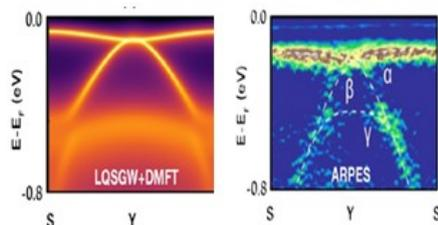
**Fig. 1:** Photoemission spectra of the high-performance low temperature thermoelectric FeSb<sub>2</sub>, theoretical prediction (left) and experimental verification (right) from Ref. 3.
