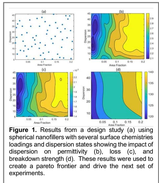
**Figure 1.** Results from a design study (a) using spherical nanofillers with several surface chemistries loadings and dispersion states showing the impact of dispersion on permittivity (b), loss (c), and breakdown strength (d). These results were used to create a pareto frontier and drive the next set of experiments.
