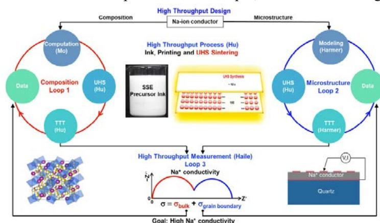
Figure 5. Closed-loop approach for materials discovery and design integrating high-throughput rapid synthesis, measurements, computation, and modeling.
