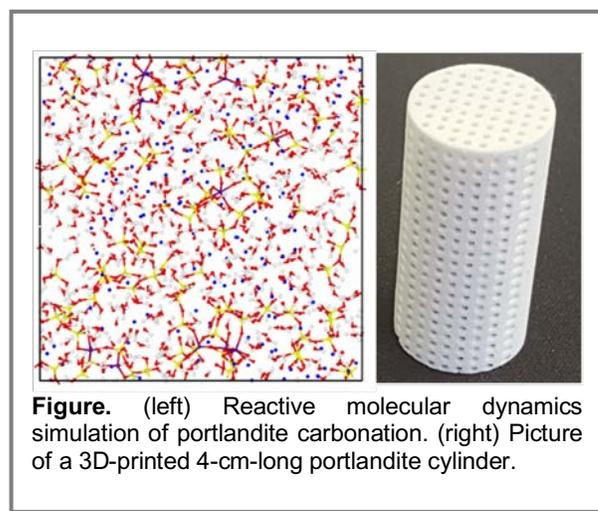
**Figure.** (left) Reactive molecular dynamics simulation of portlandite carbonation. (right) Picture of a 3D-printed 4-cm-long portlandite cylinder.
