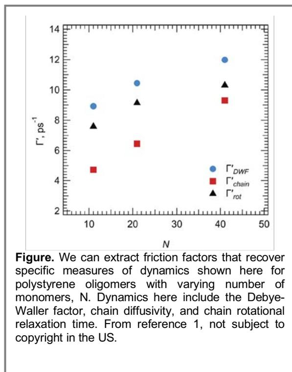
**Figure.** We can extract friction factors that recover specific measures of dynamics shown here for polystyrene oligomers with varying number of monomers,  $N$ . Dynamics here include the Debye-Waller factor, chain diffusivity, and chain rotational relaxation time. From reference 1, not subject to copyright in the US.
