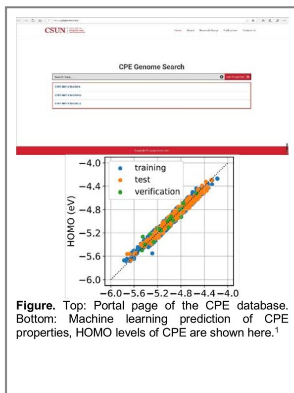
**Figure.** Top: Portal page of the CPE database. Bottom: Machine learning prediction of CPE properties, HOMO levels of CPE are shown here.<sup>1</sup>
