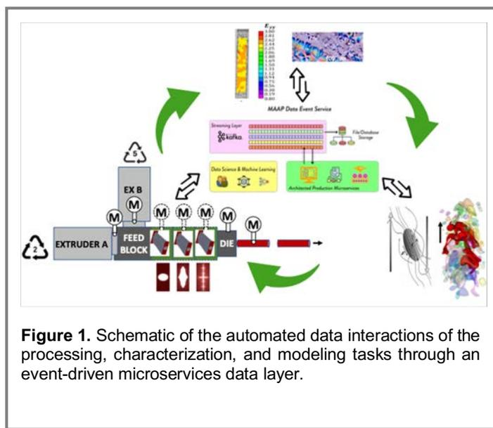
**Figure 1.** Schematic of the automated data interactions of the processing, characterization, and modeling tasks through an event-driven microservices data layer.
